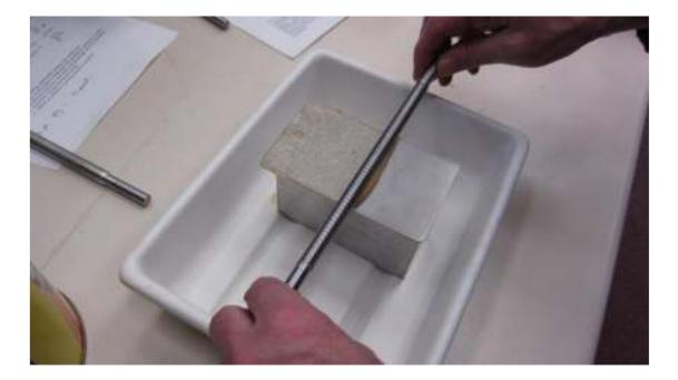
Figure 2.1 – Applying Wax with the bar coater.
