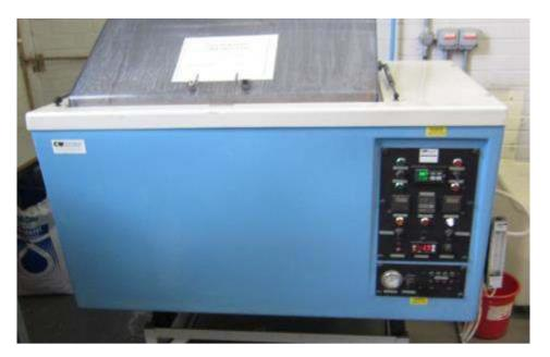
Figure 2.2.2 – Salt Spray test Chamber
